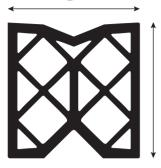
"W" is the minimum value of the gap on which the profile can be installed and this should be adjusted according to the temperature.
