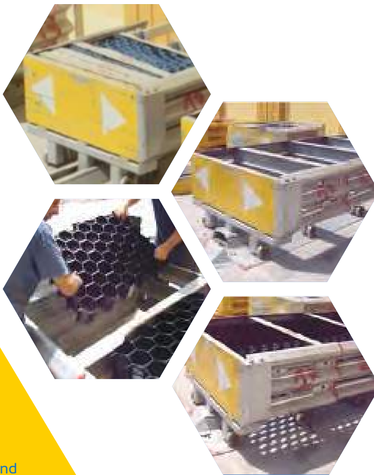
Recovery of SMA crash cushion 80 km/h after a crash test.
